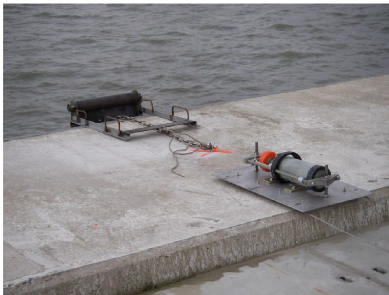
Figure 3-2: Guiding system and chain suspended from the rawlplug (left), frame with RCM-9 and steel cables (right)
