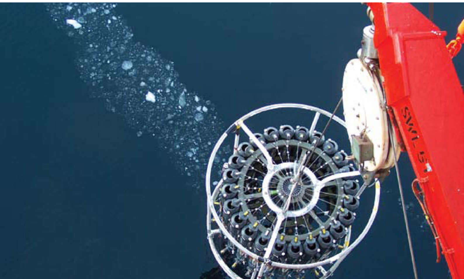
Deployment of CTD from RV Polarstern. Image courtesy of Agnieszka Beszczynska-Möller, AWI, Germany.
