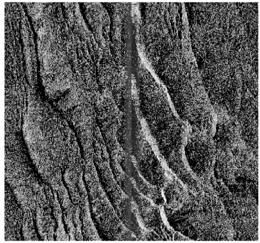
Figure A7A.3. Examples of sidescan sonar images from acoustically distinct regions. 1) Area A - Offshore clean gravel; 2) Area B Offshore gravel with thin sand veneer; 3) Area B - Offshore gravel with thick sand veneer; 4) Area C - Mega sand waves; 5) Area F - Inshore rippled sand; 6) Area E - Mixed heterogeneous sediment.
