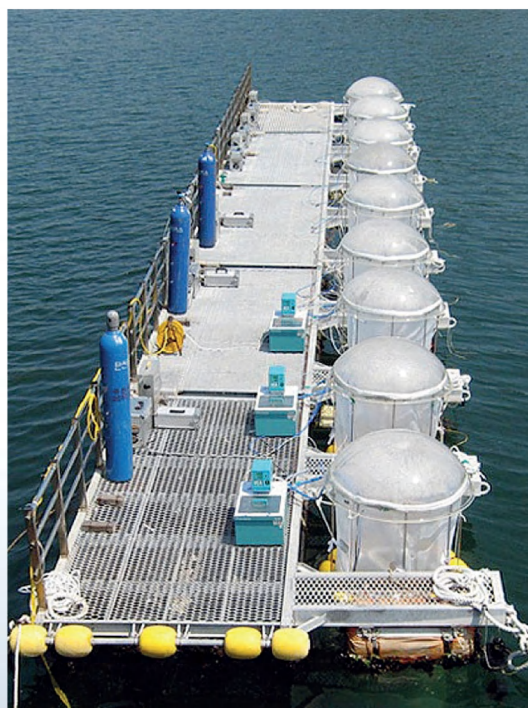
Figure 6.1 Mesocosm studies in ocean acidification research - upper left : PeECE III study in the Espegrend Marine Biological Station, Bergen, Norway (Riebesell et al. , 2008a); upper right : mesocosm facility at Jangmok on the southern coast of Korea (Kim et al. , 2008); lower panel : free-floating mesocosms deployed in the Baltic Sea (Riebesell et al. , unpubl.).
