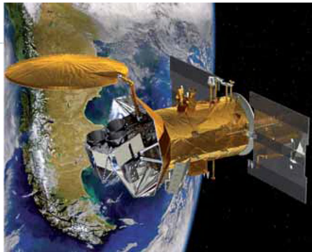
Artist's illustration of the Aquarius/SAC-D spacecraft, scheduled for launch in May 2010. It will be the first NASA instrument to measure sea salinity from space. (© Jet Propulsion Laboratories, NASA)
