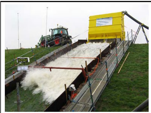
Figure 27 Recent field test in the Netherlands on the impact of overtopping waves on an existing levee.
