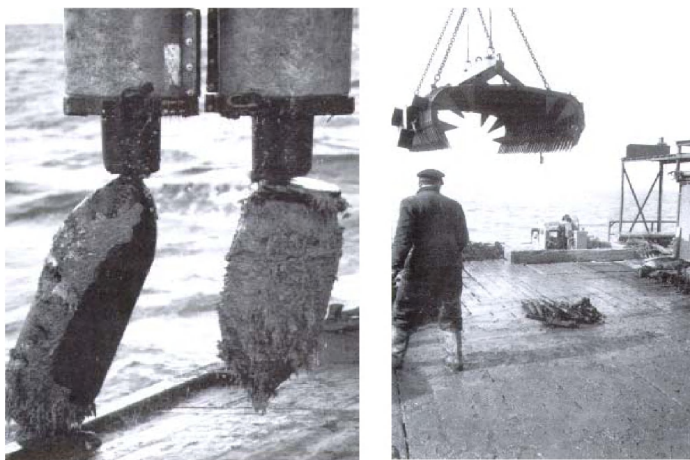
Figure 4.3 Munition recovery in the North Sea using electro-magnets (left) and large grab (right) (Rapsch & Fischer 2000).
