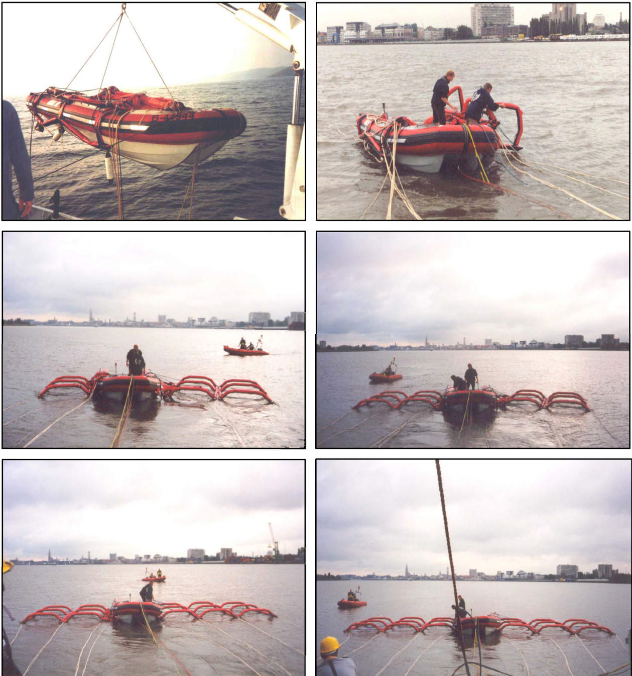
Figure 2.6 Different steps in the deployment of the inflatable array OPUS3D.
