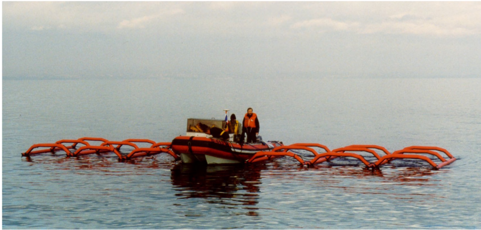
Figure 2.7 The 3D acquisition array used in stand-alone mode on Lake Geneva.
