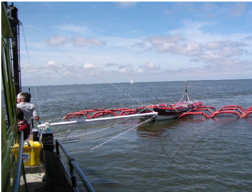
Figure 7.13 3D acquisition system on the Wadden Sea during turning. The side boom (in white) assures good stability of the outer inflatable frames
