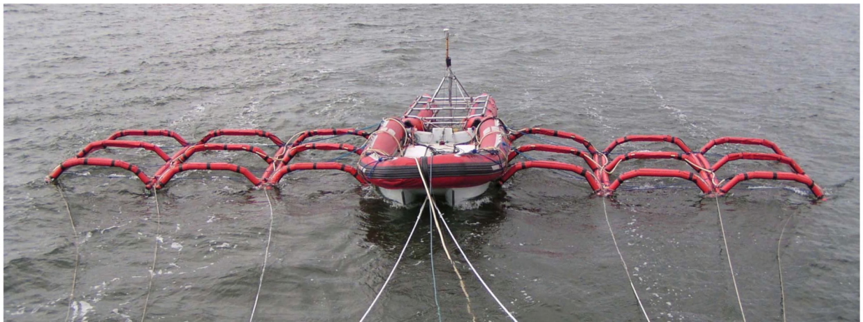
Figure 2.5 Final lay-out of the seismic acquisition system OPUS3D.
