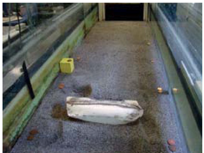
FIGURE 1a-b Bi-directional pump system and the placement of the model vessel on the mobile bed. The coins and blocks represent reference points to enable stitching of laser scans so larger surface areas can be recorded.
