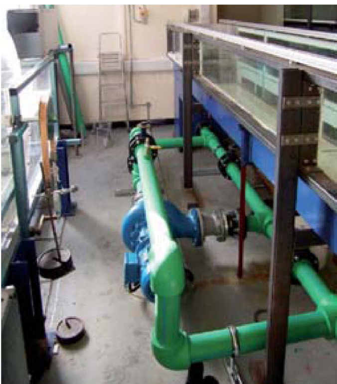
FIGURE 1a-b Bi-directional pump system and the placement of the model vessel on the mobile bed. The coins and blocks represent reference points to enable stitching of laser scans so larger surface areas can be recorded.
