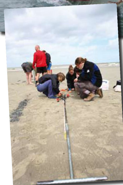
» In situ examination of a core taken on Raversijde beach (Belgium) with a Van der Staay coring device
