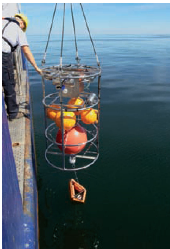
Figure 33. An underwater winch system is deployed in the deep anoxic waters of the Gotland Basin (Baltic Sea) as part of the Gotland Deep Environmental Sampling Station (GODESS) as part of the EU project HYPOX. This instrument allows high frequency and high resolution profiles of oxygen and other biogeochemical parameters throughout the water column. Such measurements are instrumental for a better understanding of coastal hypoxia. First time series results show a remarkable dynamics of the oxic/anoxic transition zone with strong implications for water column biogeochemistry and nutrient recycling. (Courtesy of Ralf Prien, Leibniz Institute for Baltic Sea Research, Germany)
