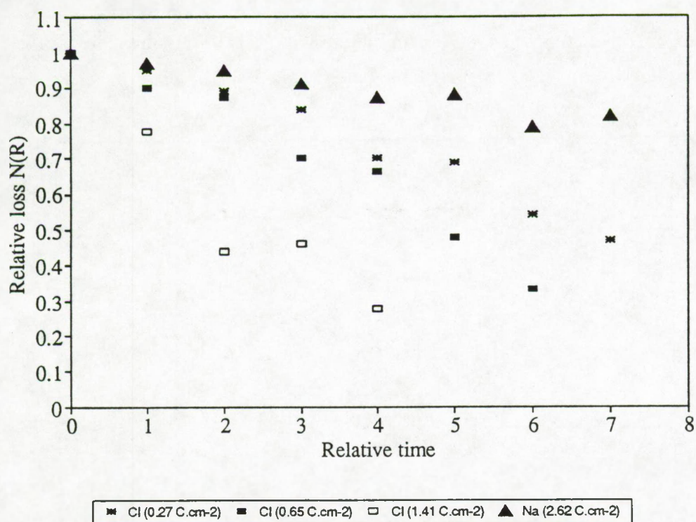
Figure 7.4: Relative loss N(R) of chlorine and sodium from NaCl as a function of time, collected at a constant electron irradiation dose. The relative loss is the ratio of the measured element intensity at constant time intervals (relative time) to the initial measured element intensity (relative time of zero).
