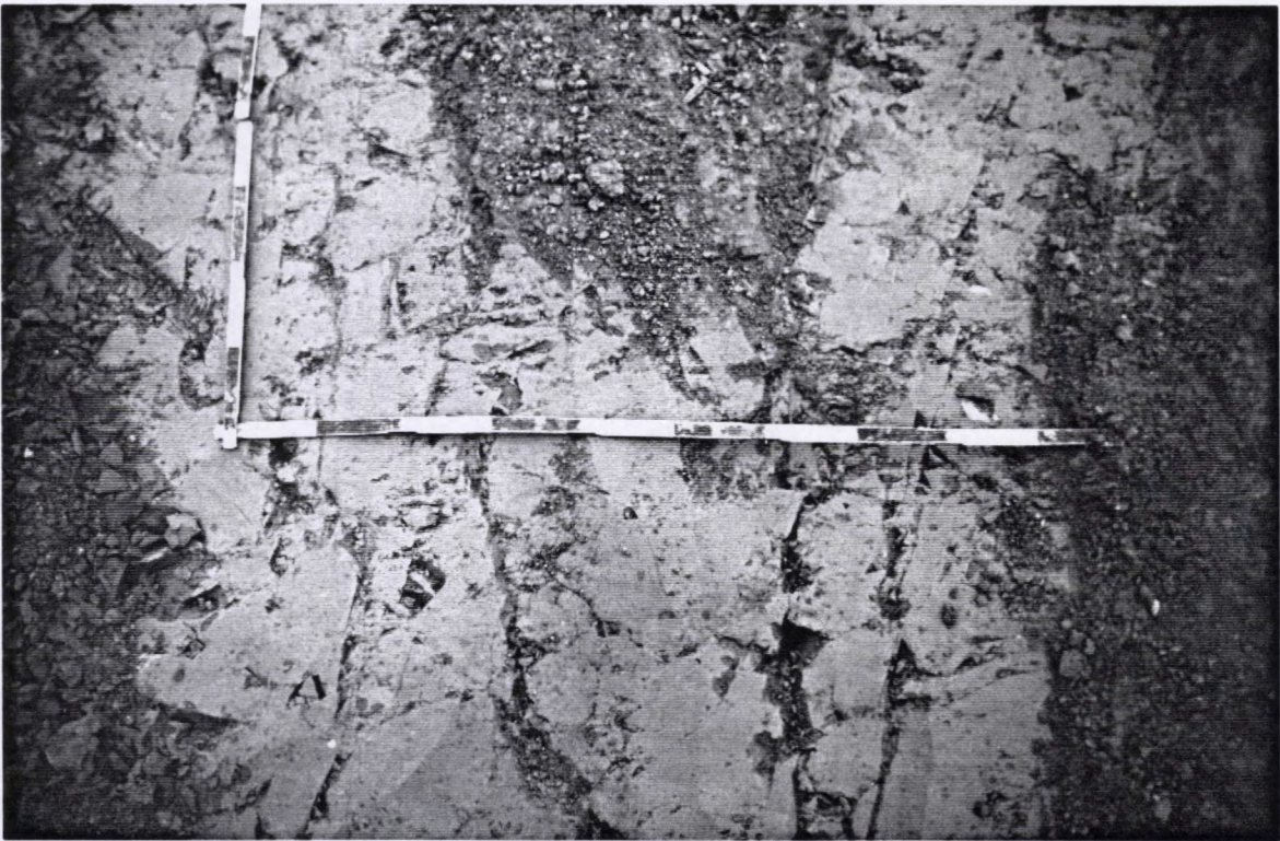
Fig. 4.19a. Clay face cleaned up. Black gouge shows up in a photograph, but not the faults, because the colour and texture contrasts are too subtle (Marke 27.10.89).
