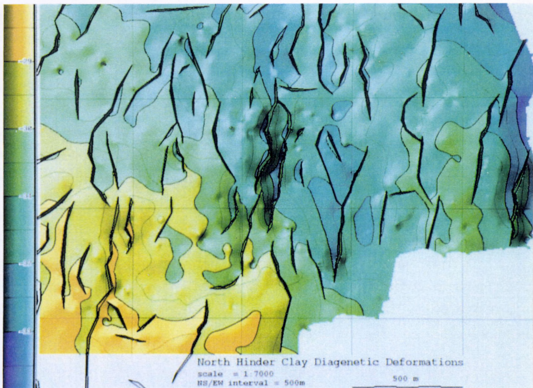
Fig. 4.5. Relief map of clay tectonic faulting in North Hinder zone (reflector indicated in fig. 2.13). Sector as in fig. 4.4; UTM grid lines every 500 m; colour interval 1 m, contour lines every 0.5 m. Fault traces in heavy black lines.
