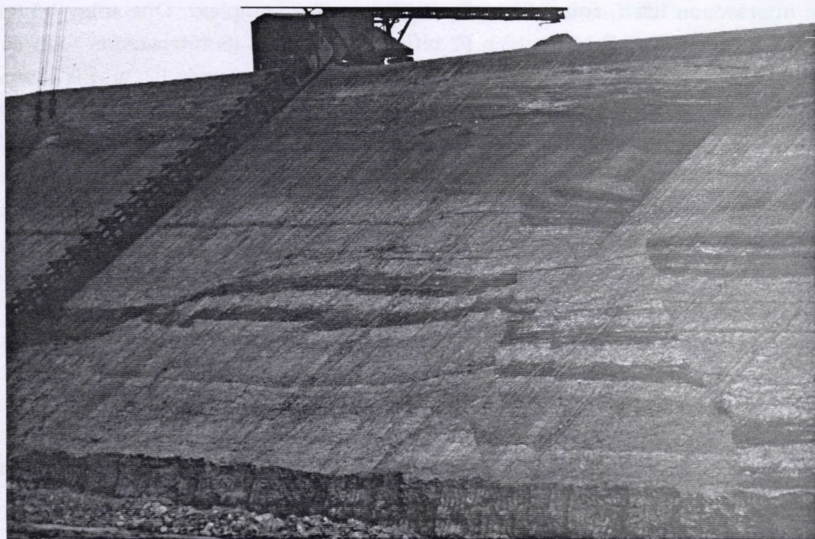
Fig. 4.25. Same view as in fig. 4.24, but one year later or about 10 m further SE. The twin faults have changed shape and a horse is now also visible on F1. The apparently low angle fault (left) intersects F1 at the top of the outcrop (Marke 01.06.88).
