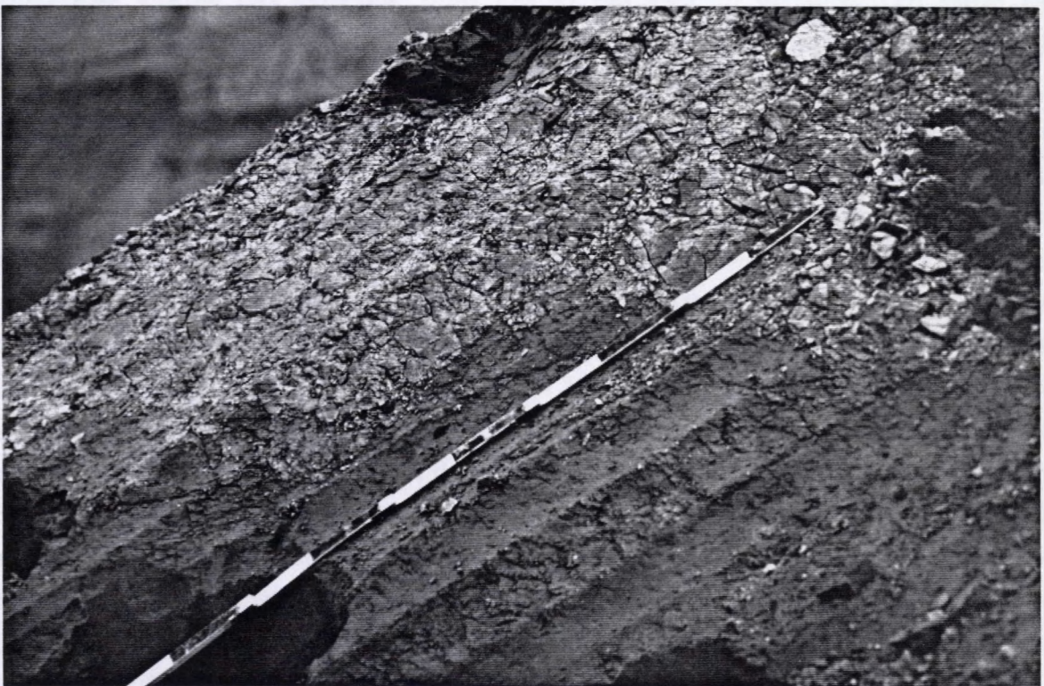
Fig. 4.15. While the clayey outcrop is drying, silts retain their grey tone. Clay, darker than silt when moist, dries to a much lighter grey colour. This colour contrast brings out bedding and faults (Marke 26.10.89).
