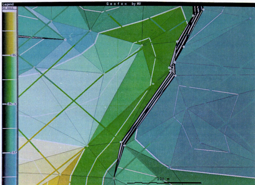
Fig. 3.26d. All fault gaps in this view are now correlated into one continuous fault scarp. Because this method uses only data points and the connections between them, alternative correlations can easily be tested. For the time being, the scarp ends on one of the sections, while it actually lies somewhere within the maze of adjacent and cross-secting horizon segments.
