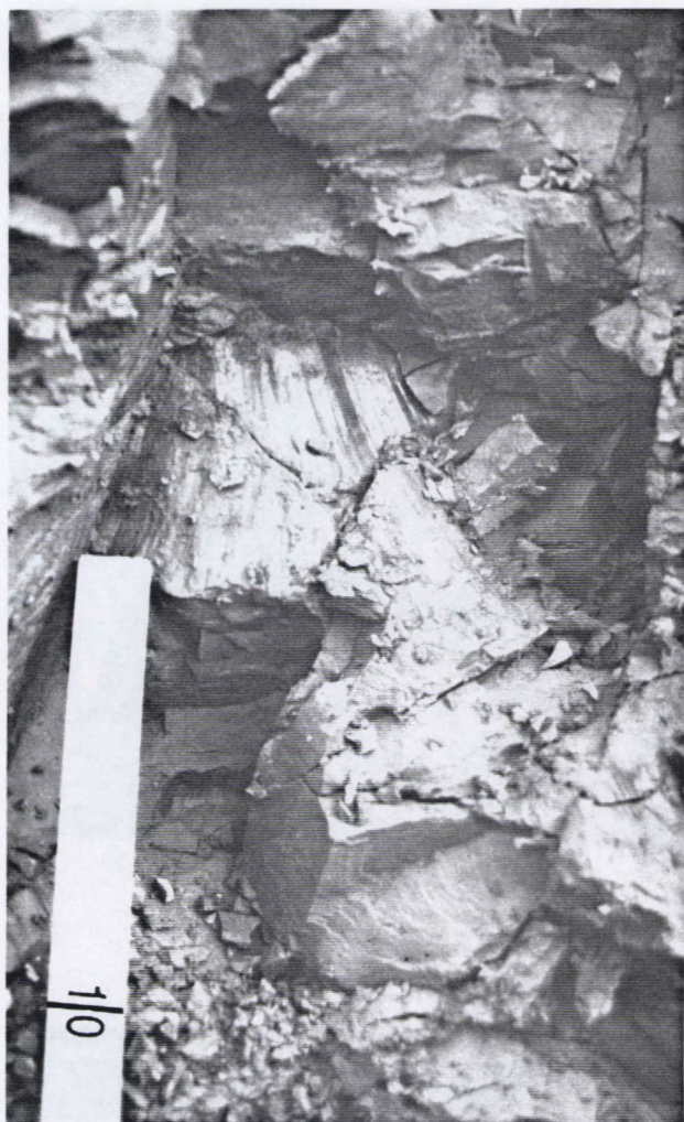
Fig. 4.43. Curved microfault with downwards diverging striae (Marke 19.10.89).
