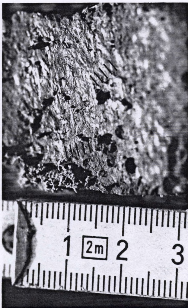
Fig. 4.41. Flat slickenside with striae in two directions (Marke 04.10.89).
