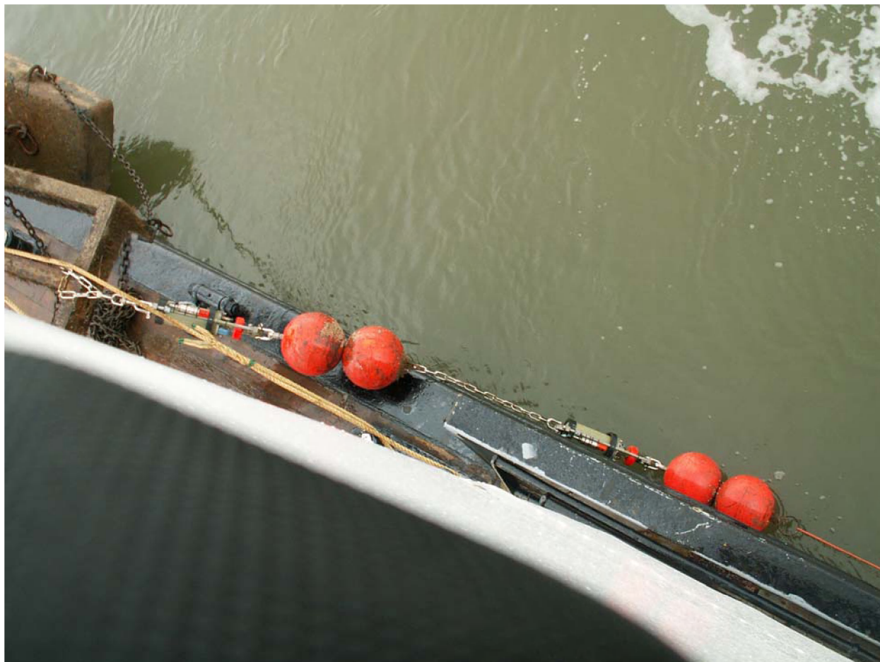
Figure 3-18: Set-up of two RCM-9 units
