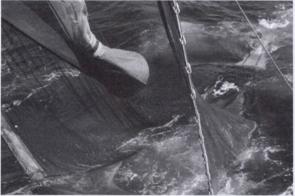
Fig. 5. The Rectangular Midwater Trawl 1+8 (RMT) deployed from the Tyro during the Netherlands Indian Ocean Programme.
