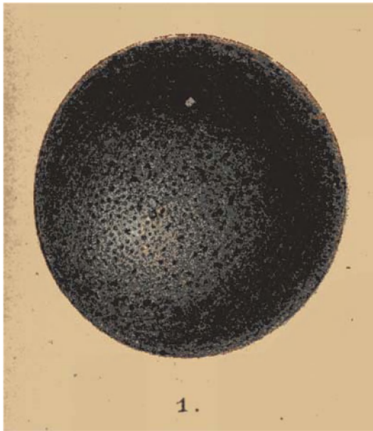
Fig. 1. Magnetic spherule of cosmic origin from Station 285; 2375 fathoms, South Pacific. This spherule was extracted from a manganese nodule, and has a coating of black magnetic iron, with a brilliant and shagreened surface (magnified 90 diameters) [313 \mu\text{m} ]
