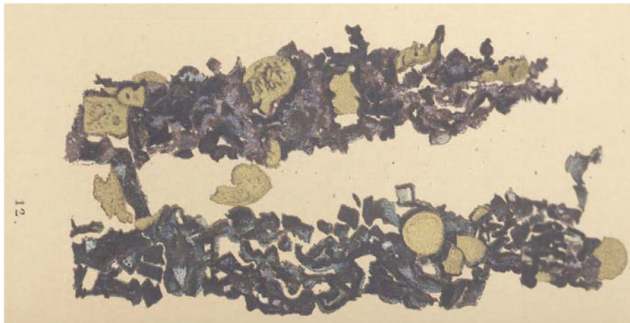
Fig. 12. Appearance of the magnetic particles extracted from Radiolarian Ooze, Station 274; 2750 fathoms, Mid Pacific, after being broken down in an agate mortar, and treated with an acid solution of sulphate of copper. The black particles are fragments of magnetite and coatings of the cosmic spherules, while those on which copper has been deposited are malleable particles of native iron (magnified 37 diameters). [ max. length =2130 \mu\text{m} ]
