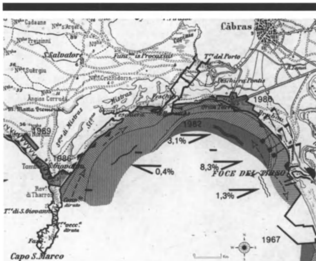
Figure 2. Subset of the map from the “Atlante delle spiagge italiane.” Map of our study area, showing the evolutionary trends of the coastline (–, stability; >, progradation; <, erosion).
