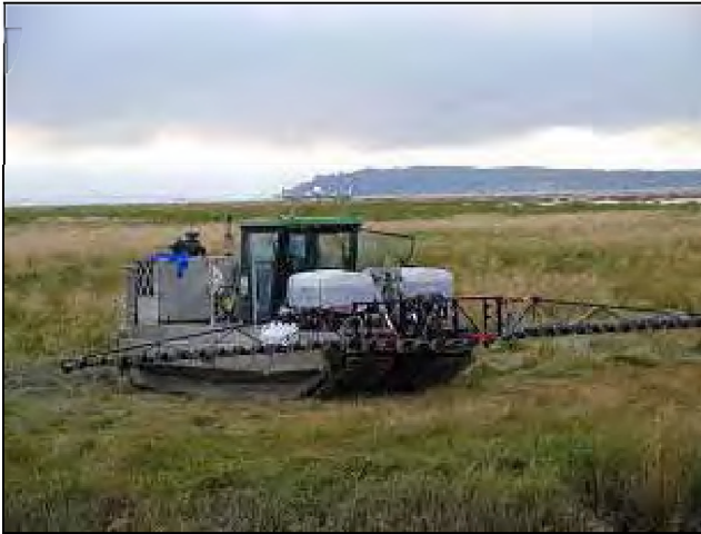
Fig. 6. Tracked amphibious machine with ground broadcast herbicide application equipment, Willapa Bay, Washington, USA.
