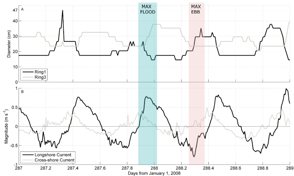
Figure 6.5 More detailed extract from the time-series data of mine rings 1 and 3 (a); and the corresponding longshore and cross-shore currents (b) for a period of 2 days (~4 tidal cycles). The currents were recorded at 3 meters above bed
