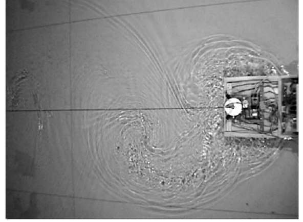
Fig. 1 Large eddies at the aft body during a test ( T=12.0 m; 10% UKC) with F_n=0.072 and n=-80\% n_0 (stopping, quadrant 2).
