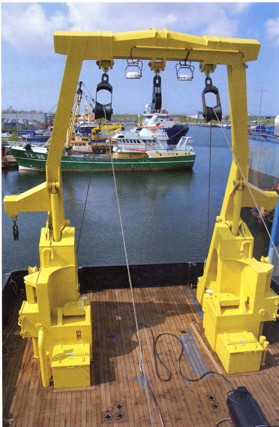
The A-frame can be used both for bottom beam trawling and pelagic fishing
