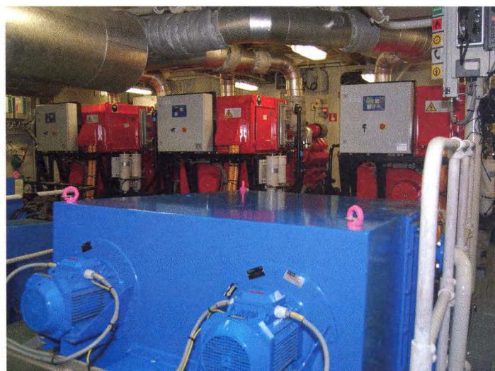
The propulsion motors are of the low-speed kind
