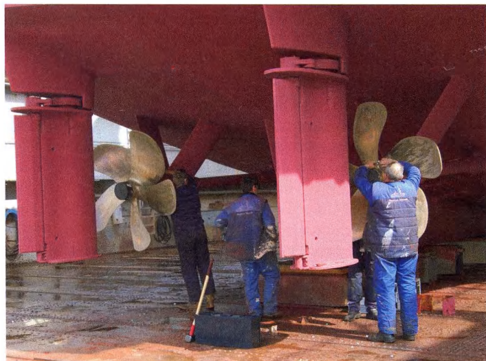
The flap-type rudders with rotary vane steering gears enable transverse thrust from the main propellers
