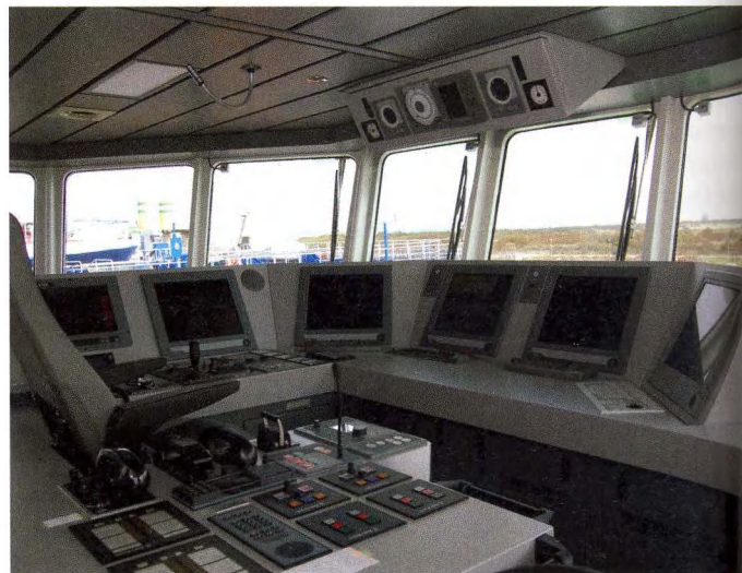
The wheelhouse features an unconventional C-shaped console
