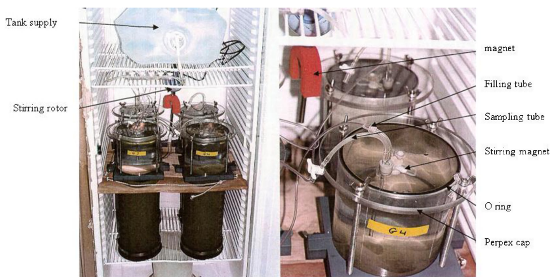
Figure 26. LABOSI assembly installed in a cooled incubator, from Denis (1999).
