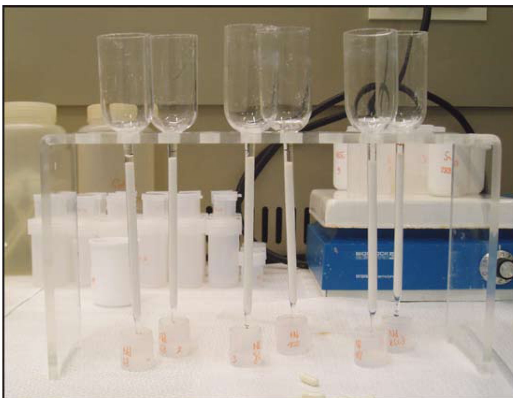
Fig. 2.14 Separation of the Nd isotopes from the other REE on a column containing Voltalef-HDEHP resin.
