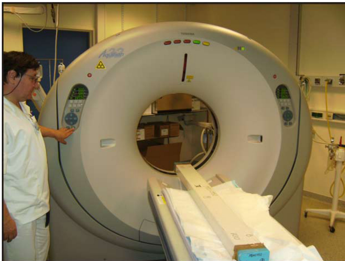
Fig. 2.4 The medical CT scanning of a sediment core in the Ghent University Hospital.
