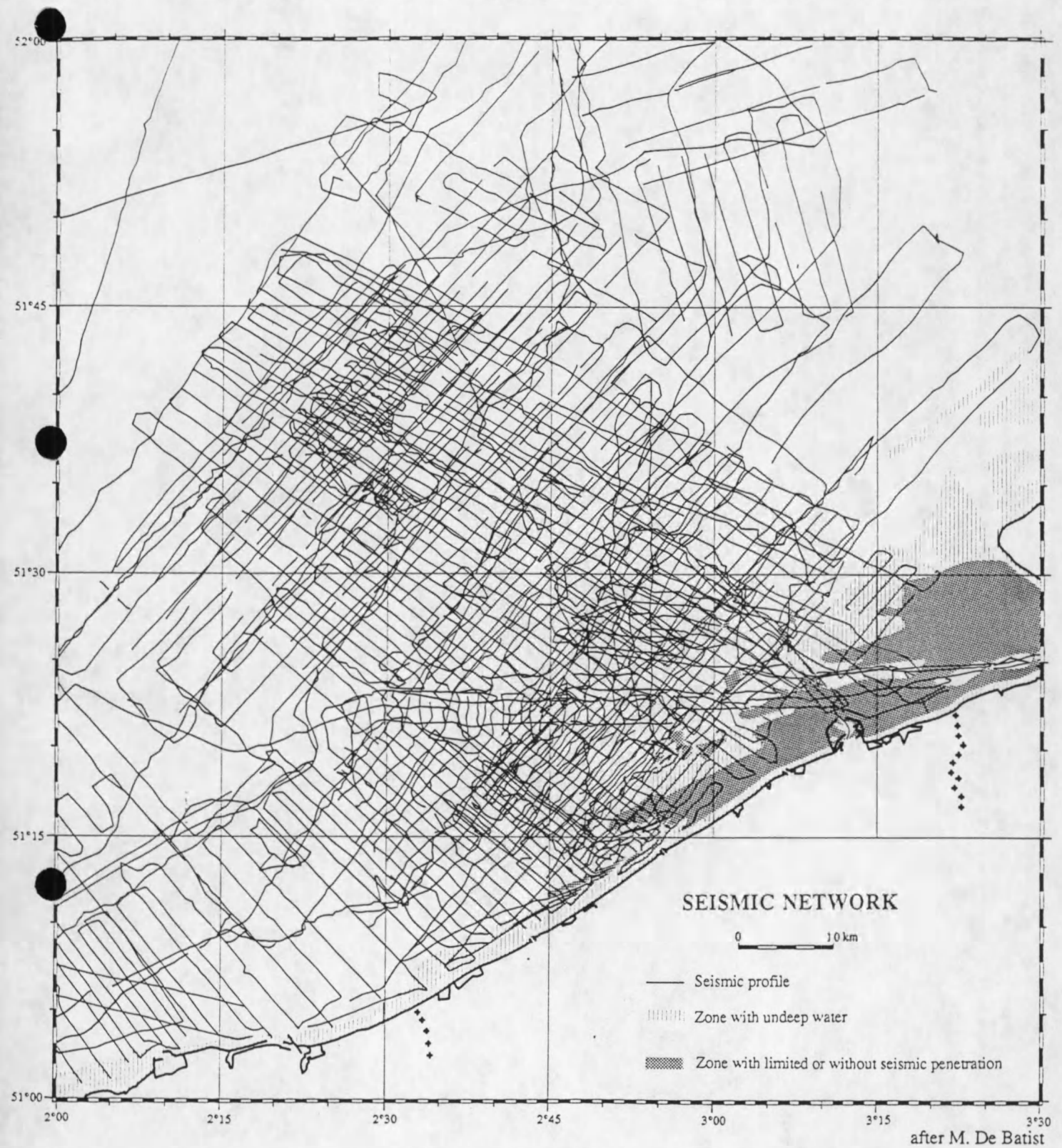
Figure 3.1 The seismic grid covering the Belgian, Dutch, French and UK sectors of the continental shelf (after Henriët et al., 1988).
