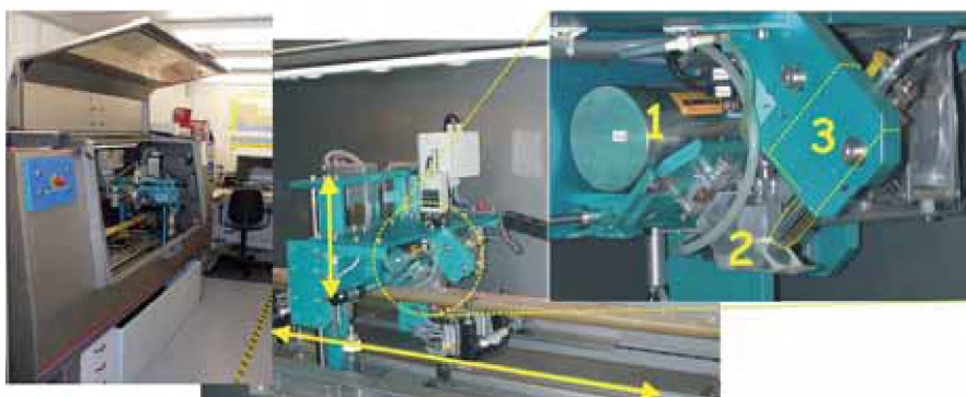
Fig. 1. Avaatech XRF core scanner at NIOZ (left) with a close-up of the XRF instrumentation (middle and right). In this configuration, the sediment surface is irradiated by an X-ray source (1) at an angle of 45°. The primary X-rays and the outgoing fluorescence radiation are transmitted through a He-flushed prism (2) to minimise diffraction and absorption. The silicon diode based detector is also mounted at an angle of 45°.
