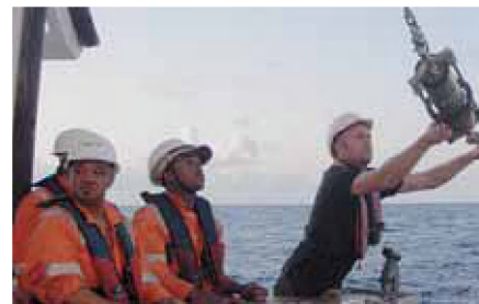
Fig. 2. Recording Current Meter (RCM) being deployed as part of one of the East Madagascar Current moorings.
