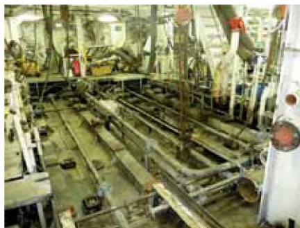
An empty engine room after removal of the generator sets.
