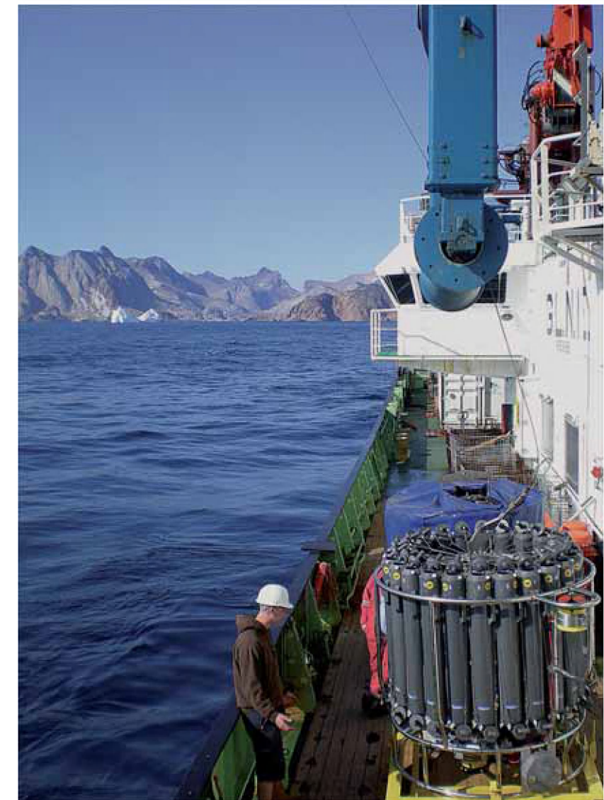
Fig. 2. The CTD ready for deployment just off the east coast of Greenland. This photo was taken on board the RRS Discovery in 2008.
