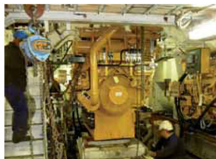
PS diesel engines brought into the engine room, due to the limited space it was a tight fit.
