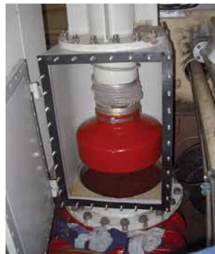
The USBL sonar head in its docking station above the gate valve
