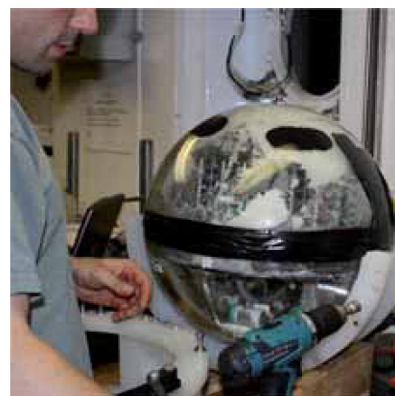
Fig. 4. Recovered National Geographic Television camera. The white material on the inside of the sphere are glass chips that broke off from the inside of the sphere.
