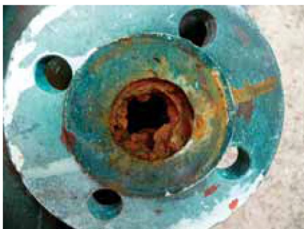
Because of the contamination in fresh water pipes they had to be renewed.
