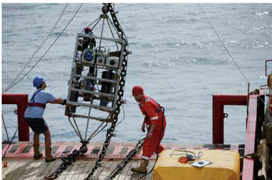
Fig. 3. The instrument cage of the surface buoy is ready for deployment.
