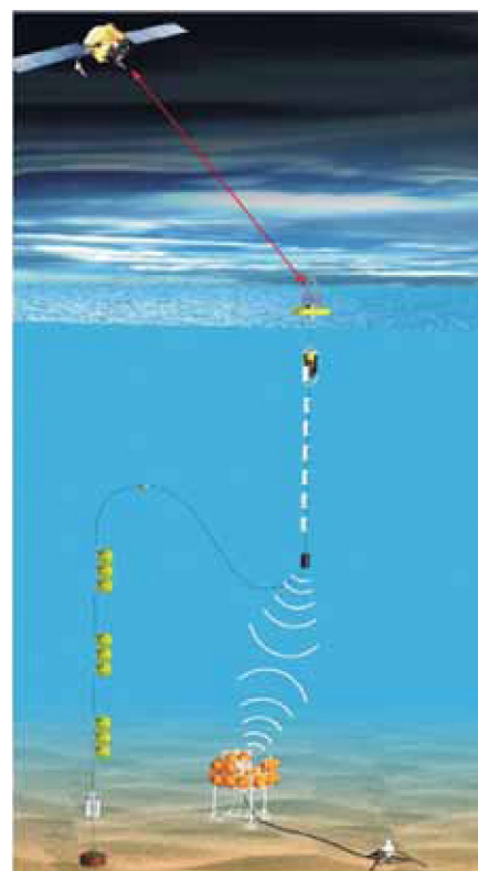
Fig. 1. Sketch of the MODOO system, where a combination of satellite and hydroacoustic telemetry enables remote control and data exchange with an observatory located on the seabed, without intervention of a deep-sea cable. Image courtesy IFM-GEOMAR, Kiel, Germany.
