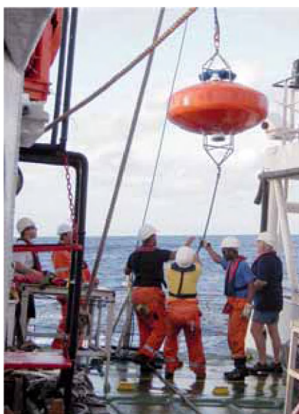
Fig. 1. Acoustic Doppler Current Profiler (ADCP) mounted inside a buoy being recovered on board the FRS Algoa in the Mozambique Channel. Facing upwards (as shown) the ADCP gathers information about the direction and speed of currents over a range of several hundred metres.
