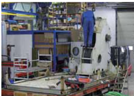
The Deep Sea Kevlar Cable winch was almost completely dissembled.....
