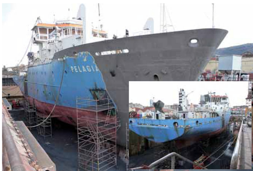
Pelagia in drydock gridblasting the hull.
