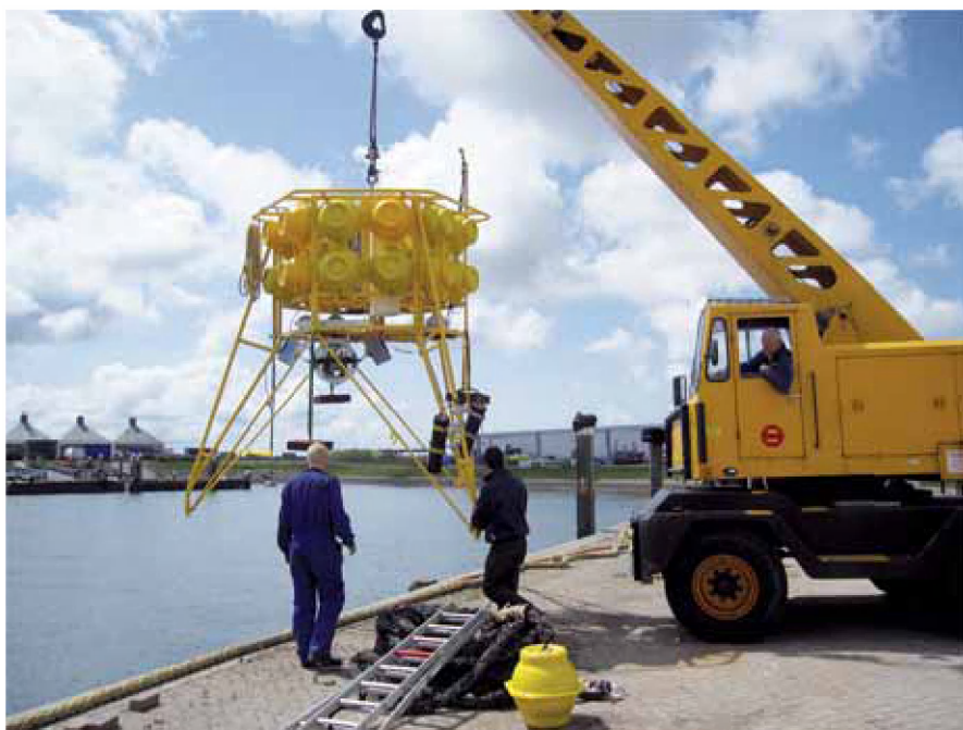
Fig. 2. Testing the BOBO lander in the NIOZ harbor.
