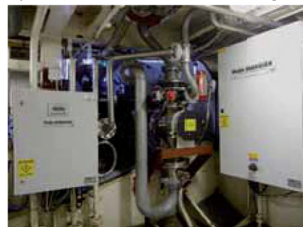
Water Ballast Treatment Unit just fits in a recess SB- Aft in the engine room.
