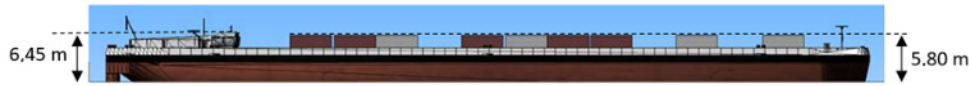
Fig. 3. Heights ship models: measured from the keel to the top of the second layer of containers (right) and measured from the keel and the top of the wheel house (left).
