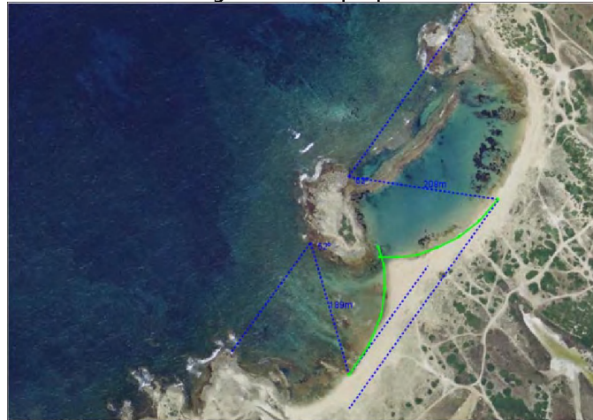
Figure 1. Standard definition sketch of geometrical properties of salients at Tuerredda beach
