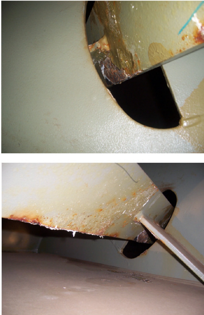
Figure 91: Effect of the presence of sacrificial anodes on the condition of the coating. Photos courtesy of Hempel.
