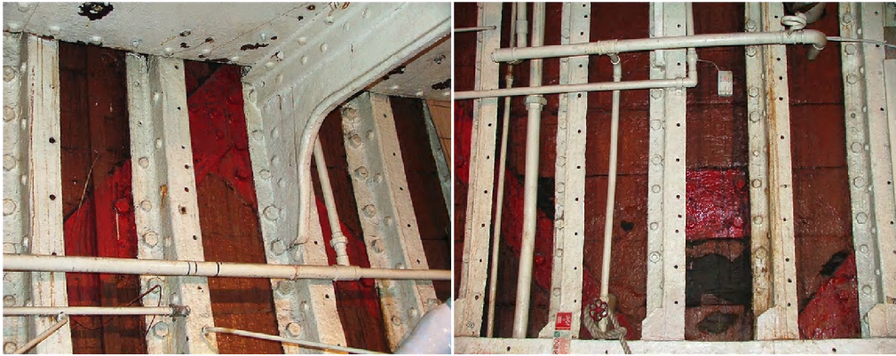
Figure 2: Composite hull structure of the Cutty Shark (Kentley, 2004)
