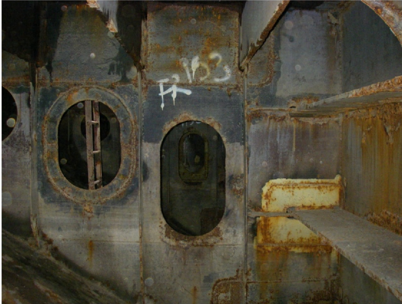
Figure 58: General corrosion in the ballast tanks of the Algoma Guardian, 25/09/2009
