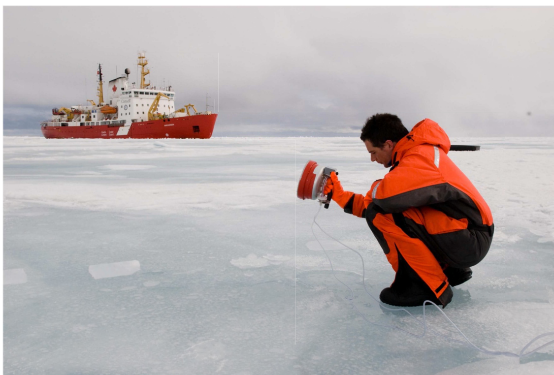
CO 2 fluxes measurements over sea ice (using chamber of accumulation), CCGS Amundsen in the background
