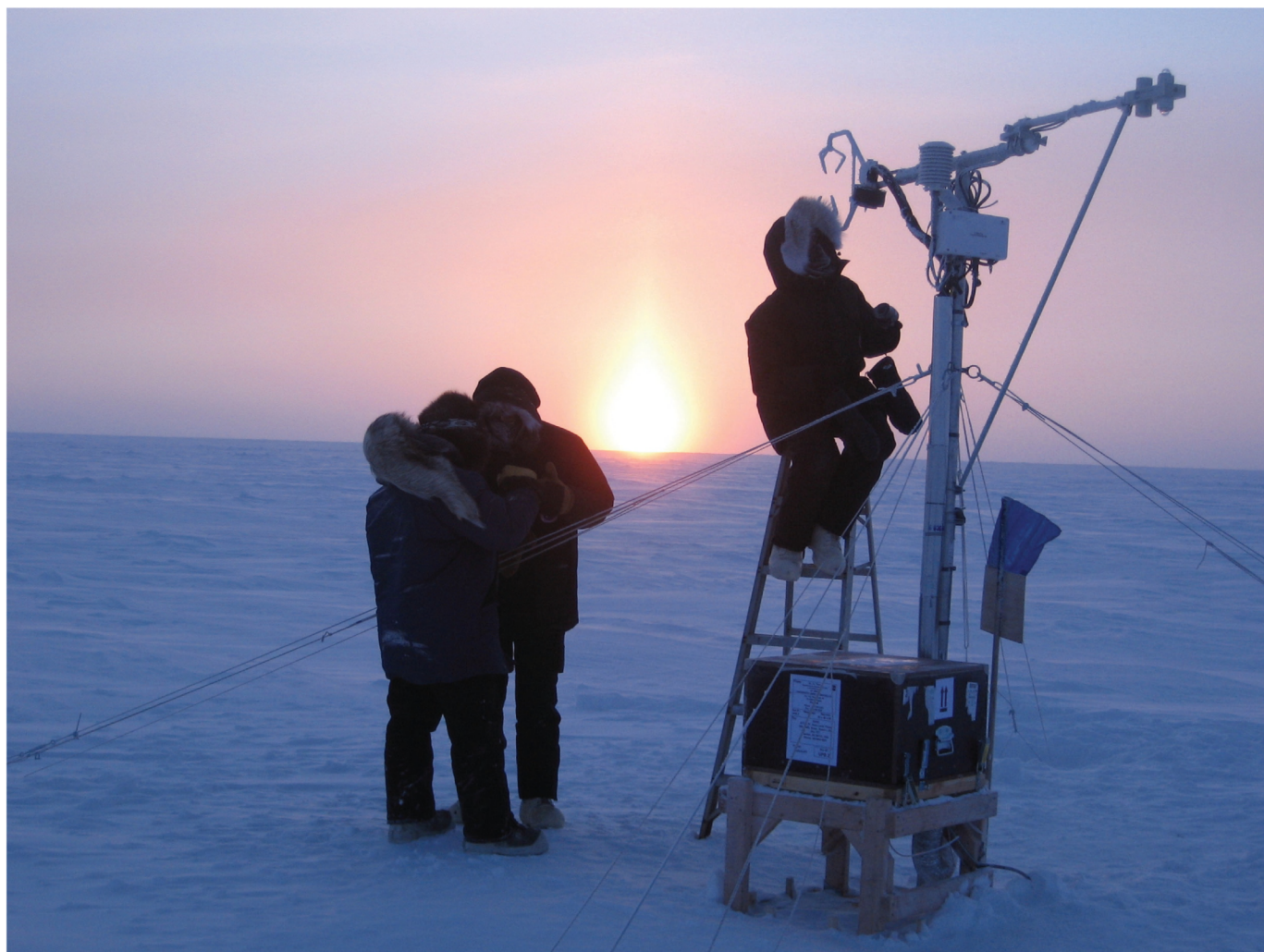
Figure 1: Set up of the mast with sonic anemometer, air intake of the CO 2 analyser and radiometer over sea ice near Barrow (Alaska) in January 2009. The temperature was -35°C.
