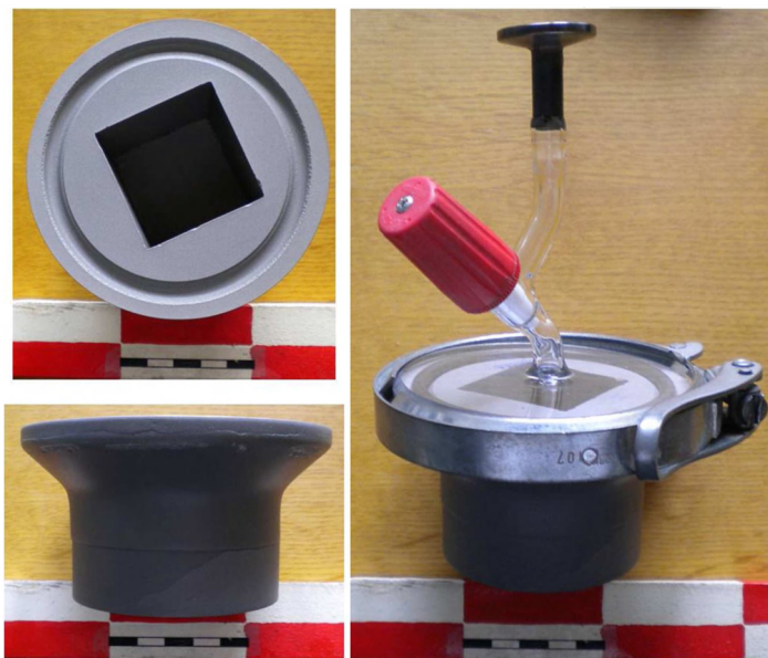
Figure IV.1: Dedicated container for the measurement of pCO 2 in solid sea ice samples, equipped with a flat glass top, silicon joint and a clamp.
