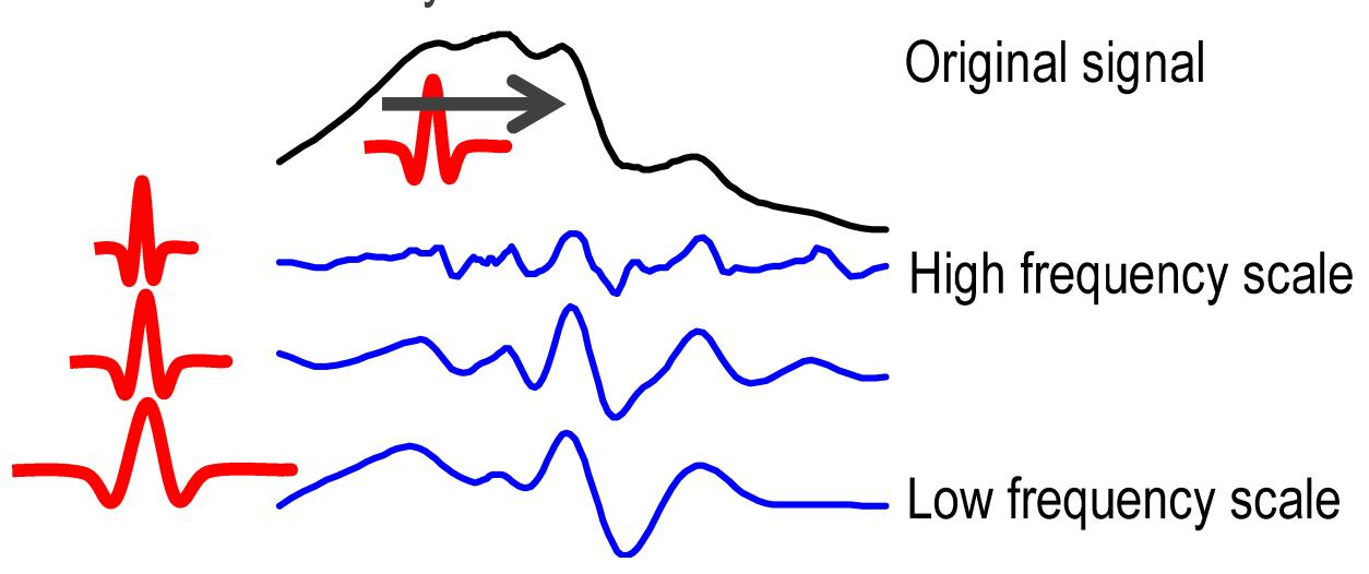
Scales are obtained by convolving the signal and the filter Each time the filter is shifted and scaled
