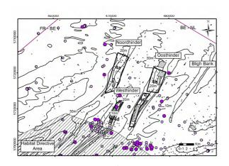
Figure 1. The Belgian part of the North Sea (a) and the area of the Hinder Banks (b), where intensive marine aggregate extraction is allowed in 4 sectors (black polygons). A Habitat Directive Area is present at a minimum of 2.5 km from the southernmost sectors. The size of the dots represents relative amounts of gravel with a minimum of 20 %. Borders with France (FR-BE) and the Netherlands (BE-NL) are indicated. In the grey shaded areas repetitive multibeam recordings.
