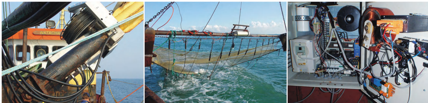
Components of the HOVERCRAN system include (l to r) the electric winch, the adapted beam trawl, and the control cabinet.
