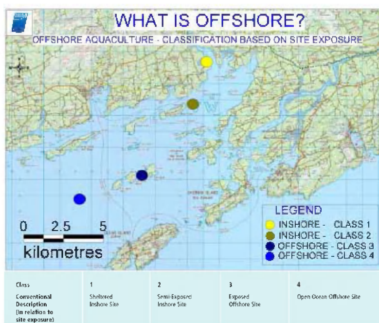
Figure 4.1. Site classification as a definition for the term "offshore" (modified after Ryan 2004).
