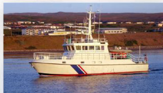
M/V Barður was built as a custom survey vessel for the Icelandic Coast Guard – Hydrographic Department in 1991. The vessel is 21 meters long, 5 meters wide and is fitted with RESON multibeam echo sounder.
