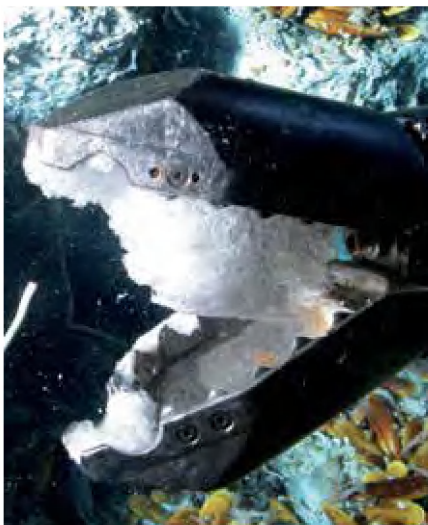
IFREMER ROV (Remotely Operated Vehicle) Victor 6000 taking samples of gas hydrates at 3,200m water depth off the Congo margin, Gulf of Guinea.
