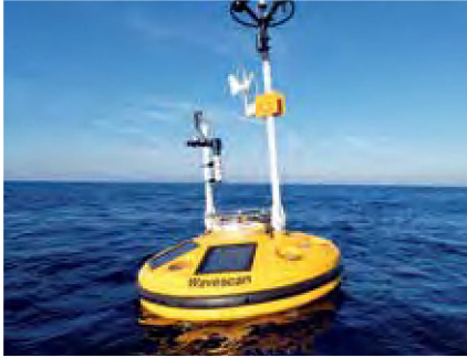
Ocean buoy and mooring for fixed-point measurements
