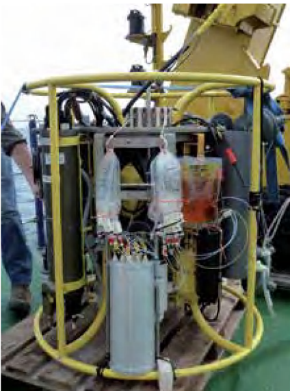
Iron and manganese sensor in insulating case, attached to CTD-Pump carousel, ready for deployment in the Baltic Sea (IOW, Warnemunde, Germany).
