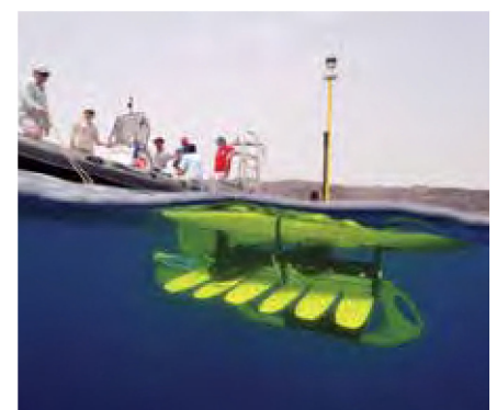
A Wave Glider just before the launch bundle is released. The Wave Glider SV Series are the first unmanned autonomous marine robots to use the ocean's endless supply of wave energy for propulsion
