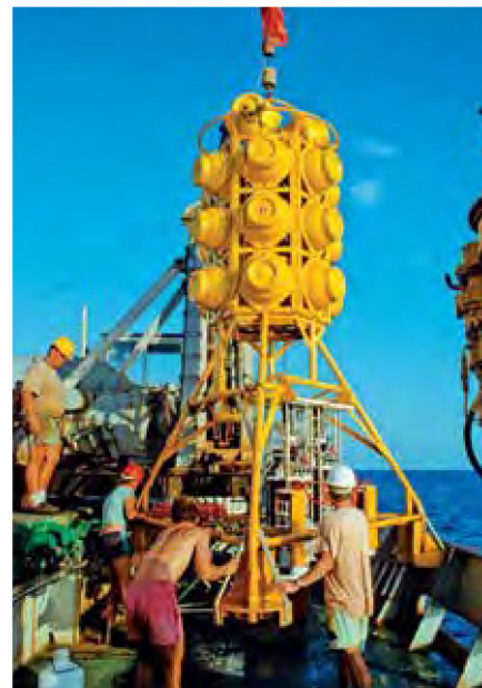
Albex Lander used for seafloor observation
