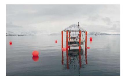
2.5 > In order to determine the effect of increasing atmospheric CO<sub>2</sub> concentrations on the ocean, an international research team enriched seawater with CO<sub>2</sub> in floating tanks off Spitsbergen, and studied the effects on organisms.
