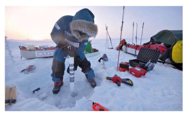
2.6 > By studying ice cores scientists want to discover which organisms live in the ice. Air bubbles in Antarctic ice cores also provide clues to the presence of trace gases in the former atmosphere, and to past climate. The ice cores are drilled using powerful tools. For more detailed study they are analysed in the laboratory. When ice crystals are observed under a special polarized light, their fine structure reveals shimmering colours.
