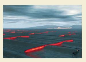
7.12 c > The Pelamis wave energy transformer floats on the ocean like a giant sea snake. It consists of several segments which move against each other and build up hydraulic pressure. This in turn drives a turbine. A new Pelamis generation is currently under construction.
