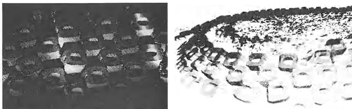
Figure 1. Images of the armour layer of the Ostend breakwaters created using terrestrial lidar.
