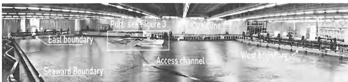
Figure 2. Overview of the large physical model. The coastline measures 55 m and the west boundary 35 m. The strong flood flows go from West to East across the access channel.
