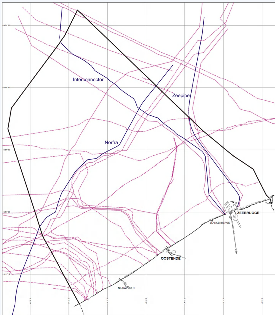
Figure 5. The cables and pipelines (in blue) in the BNS ( Continental Plat & Vlaamse Hydrografie 2013 227521 ).
