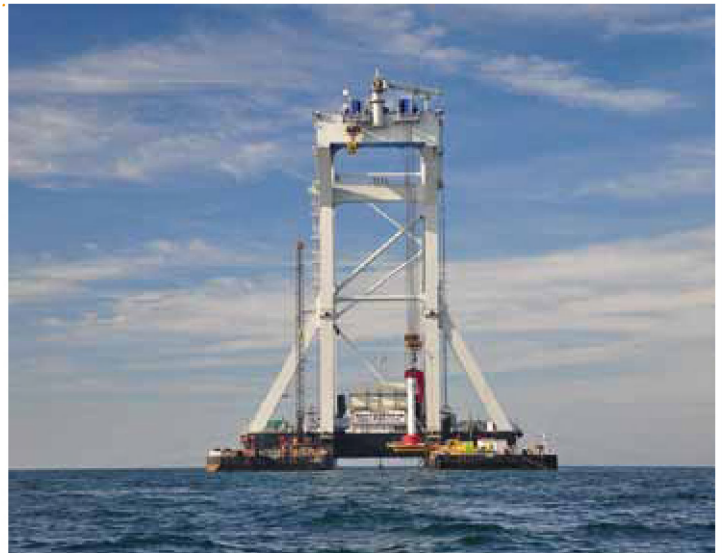
Piling vessel (with red and white hammer) at the Belwind site on the Bligh Bank.
