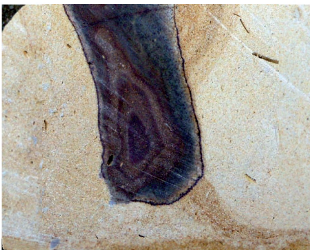
Fig. 10. 'Elst tauw' from St Servatius church at Sluizen: cut surface (width of flint nodule 3 cm) in light yellowish brown silicified mouldic bioclastic limestone containing elongated, purplish zoned flint nodule. Matrix silicification provides strong bond between original flint and surrounding tauw (RBINS building stone collection 222).
