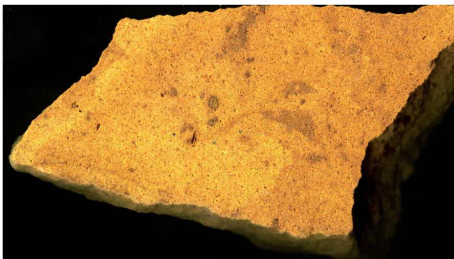
Fig. 6. 'Elst tauw' from the Maurissen sand pit: cut surface (largest diameter 10 cm) in orange brown, strongly porous 'vuggy' silicified calcarenite with frequent moulds of dissolved fossils (thin shells, serpulids, cidarid echinoid), displaying pedogenic weathering (R. Meuris Collection).
