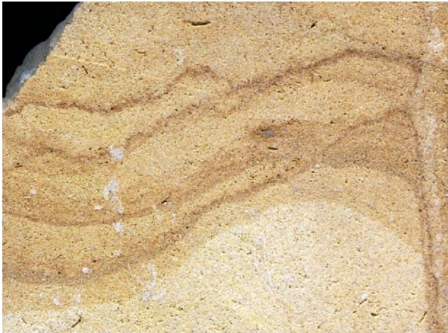
Fig. 9. 'Elst tauw' from St Servatius church at Sluizen: cut surface (width 10 cm) in creamy-white silicified mouldic-bioclastic limestone, still containing calcitic allochems, displaying brown Liesegang rings which concentrate iron and insolubles, possibly developed after extraction (RBINS building stone collection 222).
