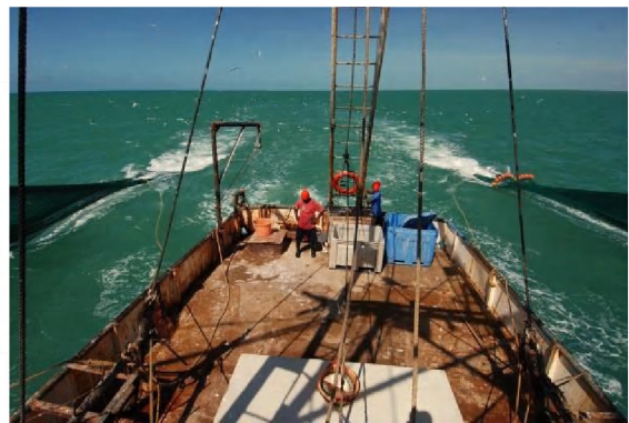
Figure 3. Simultaneous catch-comparison hauls comparing the test-net (r.) to the control-net (l.) ©Tomas Willems/ILVO
