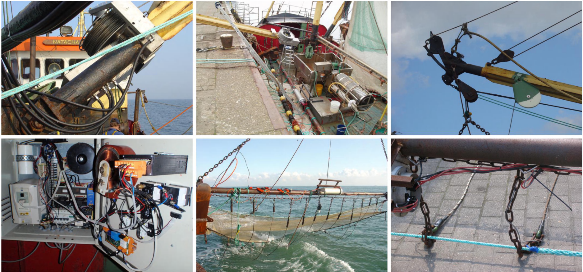
Figure 10: Detailed photographs of the installed HOVERCRAN system. Top left: Electric winch; top middle: Deck infrastructure; top right: Additional pulley block guiding the supply cable; Below left: control cabinet; Below middle: the adapted shrimp beam trawl; below right: Electrodes
