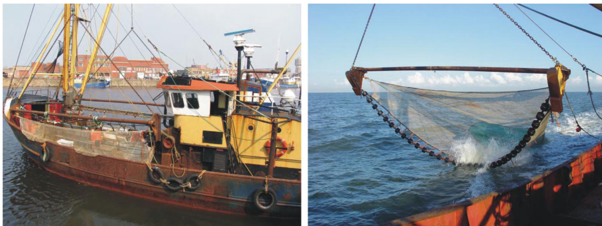
Figure 1: Left: Traditional brown shrimp beam trawler; Right: Traditional beam trawl with heavy bobbin rope
