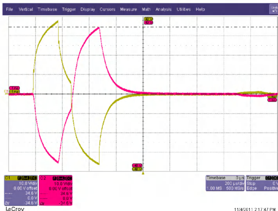
Figure 21 Electrode voltage measured on 4 November 2011 on-board OD17 on the latest HFK electrode design across the most frontal 27 mm conductor (electrode is built of 2 conductors of 27 mm and 10 conductors of 33 mm diameter). Channel 1 represent the pulse across the frontal conductors, Channel 2 the pulse at the back end of the electrode, respectively 38 and 34 V.
