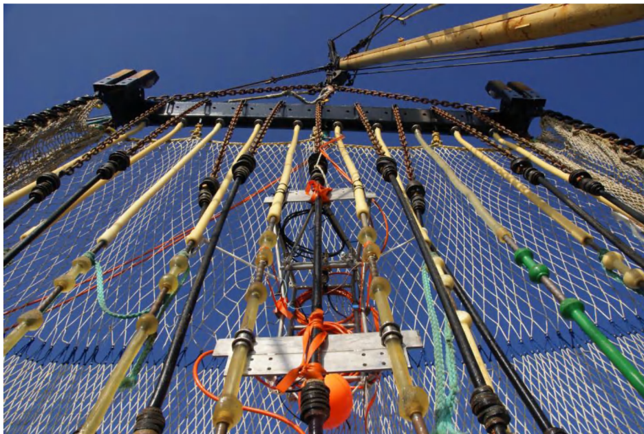
Figure 18 The rigid frame carrying three field strength probes and an DeepSea 1060 underwater video camera clamped on the first conductor pair of field 5 of the Delmeco pulse system on-board TH10 (220 kW licenced vessel).
