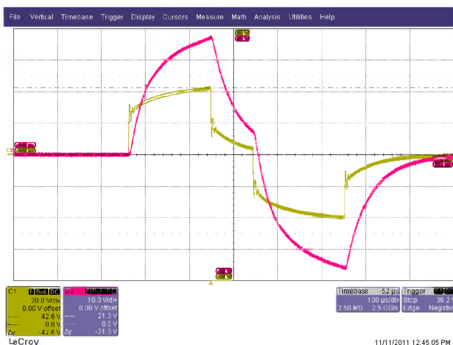
Figure 22 Electrode voltage measured on 11 November 2011 on-board OD17 on the previous HFK electrode design across the most frontal 27 mm conductor (electrode is built of 12 conductors of 27 mm). Channel 1 represent the pulse across the frontal conductors, Channel 2 the pulse at the back end of the electrode, respectively 42.6 and 37 V.
