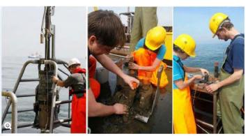
Cefas (UK) provided a Sediment Profile Imaging (SPI) camera to take photos of the sediment profile form which sediment function can be inferred.
