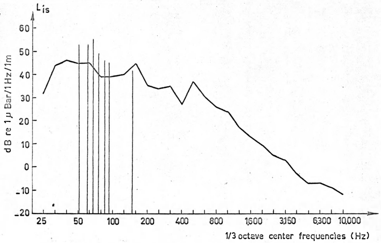
Figure 5 - Sound spectrum of the main engine idling at 1150 rpm
