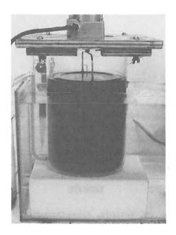
Fig. 1. Continuous dilution system simulating dispersion of a treated oil slick.
