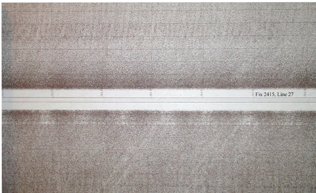
Photo 5 Lag gravels with sand streaks. (Horizontal scale, 100m between vertical fix marks; vertical scale, 12.5m slant range between horizontal lines.)
