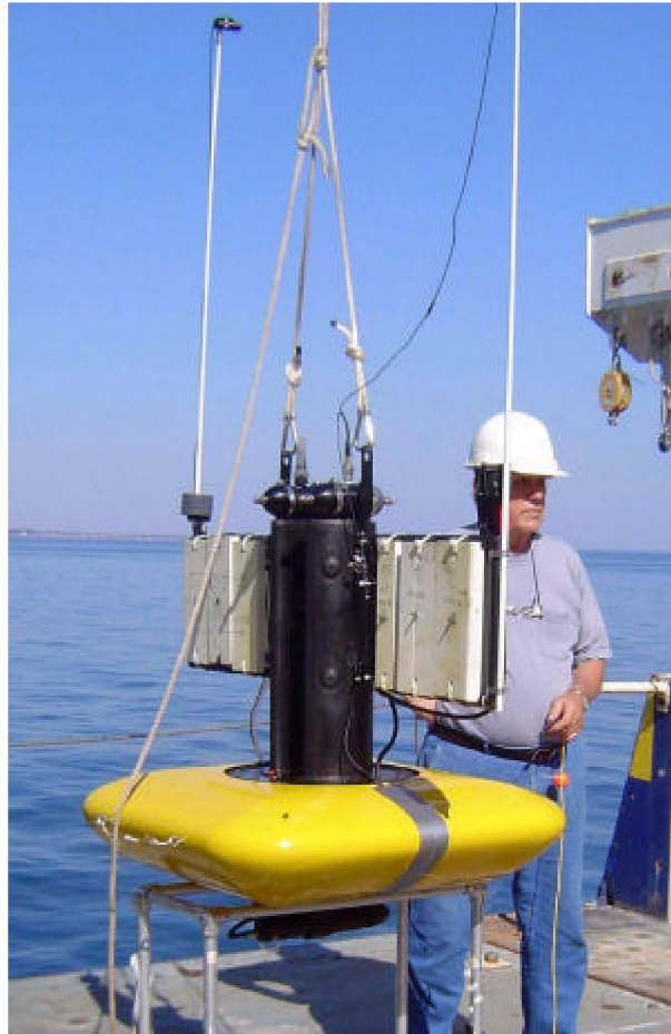
Fig. 7. Holographic camera, developed at the John Hopkins University (Maryland, USA), on board IFREMER RV Thalassa during the HABIT 2006 cruise (Photo: W. Pfitsch).
