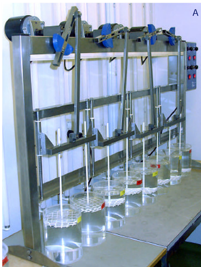
Fig. 13. Examples of two commonly used setups to generate turbulence in the laboratory. (A) The FERMETA system is used to generate turbulence in 2 l containers by means of vertically oscillating grids for laboratory experiments with plankton. FERMETA has a modular setup with 4 independent variable frequency AC gear-head motors in the standard design. Each motor may have a different nominal rotation speed, which can be reduced to 1/20^{\text{th}} through a frequency controller. Thus, the setup allows for 4 different levels of turbulence to be tested simultaneously (2 replicate containers per motor) overcoming initial conditions variability. The container lids have a sampling port to introduce a glass tube attached to silicone tubing that allows withdrawing samples by gravity (Photo: F. Peters); (B) Couette cylinders: the relevant parameters and variables to calculate \mathcal{E} are the radii of inner and outer cylinders ( r_i and r_o , respectively) and their angular velocities ( \Omega_i and \Omega_o , respectively) and the height of the cylinder ( h ) (modified from Berdalet and Estrada, 2005).
