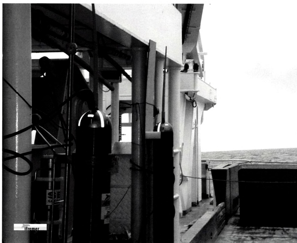
Figure 1. Two temperature PROVOR profilers on board LA THALASSA before launching. One profiler is linked to a reference CTD for metrological comparisons (photo S.Le Reste - IFREMER).
