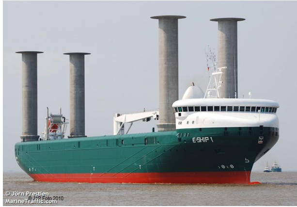
(a) The E-Ship 1, manufactured by Enercon and equipped with 4 Flettner rotors [57].
